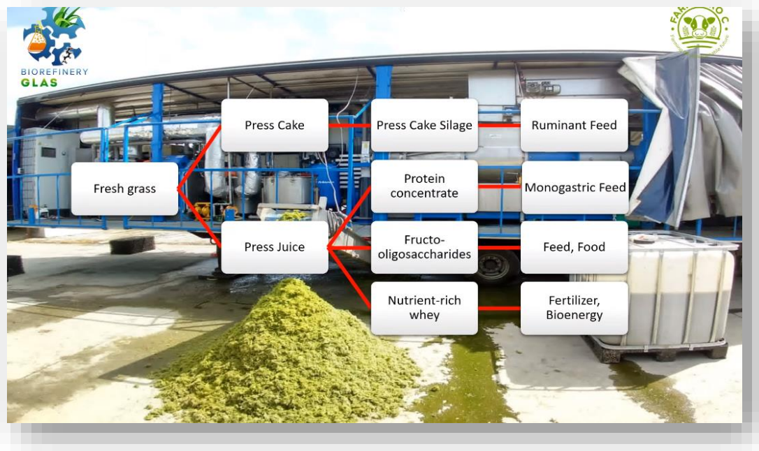
Fig 6: Fresh grass is separated into press juice and press cake; juice yields protein concentrates and functional carbohydrates; cake and brown juice go to AD; digestate returns nutrients to soil; biomethane and CO 2 support energy/users 116 .
